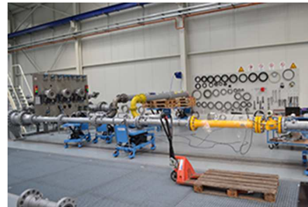
Test results of Energoflow GFE 404 at RMA calibration facilities (two bends in different planes + half-moon opening, air, natural gas) 2017 yr
