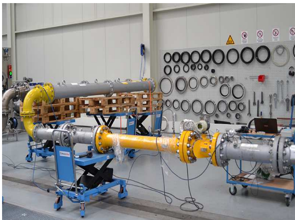
Test results of Energoflow GFE 404 at RMA calibration facilities (standard conditions, air, natural gas) 2017 yr
